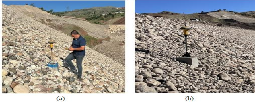
Figure 2.a-b: GPS readings at external benchmark points
