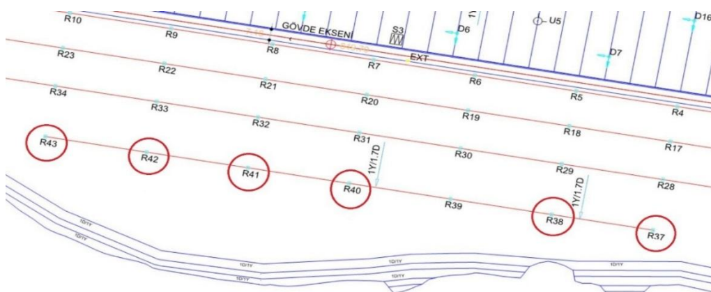
Figure 1. External Benchmark Points Layout Plan
