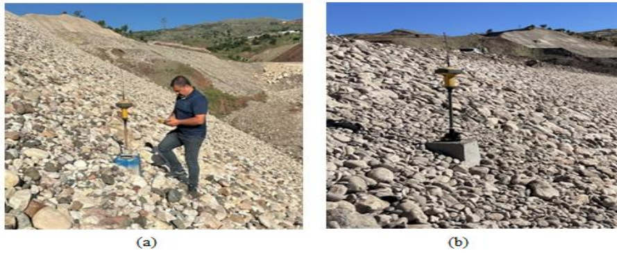
Figure 2.a-b: GPS readings at external benchmark points
